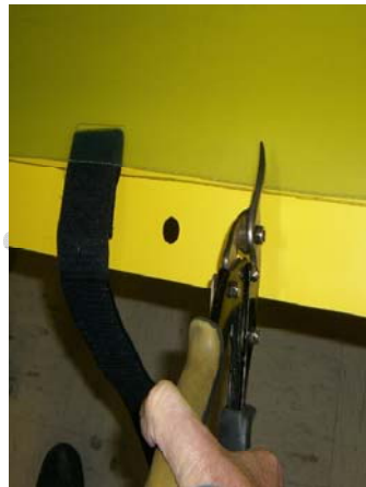
Cut down sheet to fit inside hatch if necessary.
